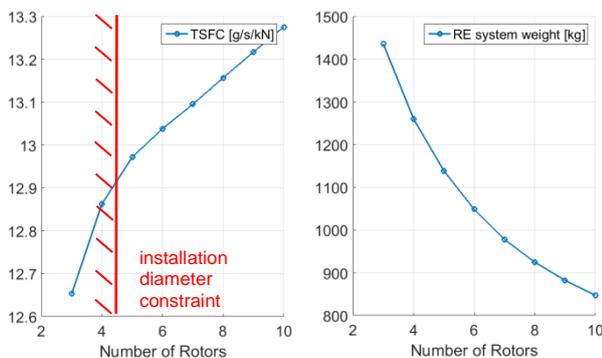
FIG 6. Thrust specific fuel consumption (left) and RE system weight (right) for different numbers of RE rotors
