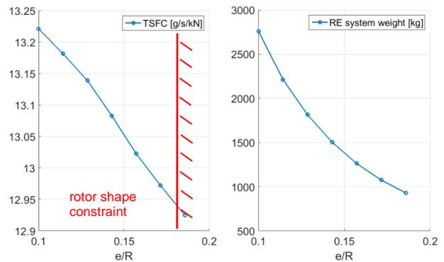
FIG 5. Thrust specific fuel consumption (left) and RE system weight (right) for various  $e/R$ -ratios
