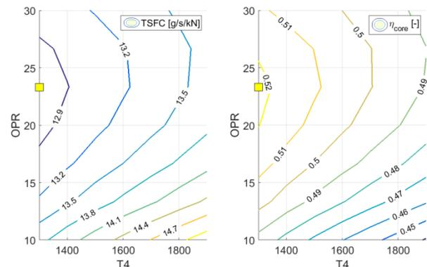
FIG 7. Thrust specific fuel consumption (left) and core efficiency (right) for T4-OPR study
