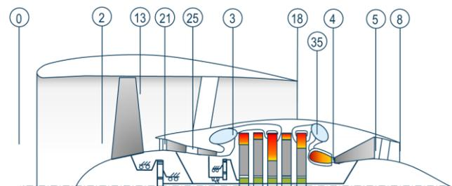
FIG 2. Basic conceptual sketch of a CCE with coaxial rotary internal combustion engine
