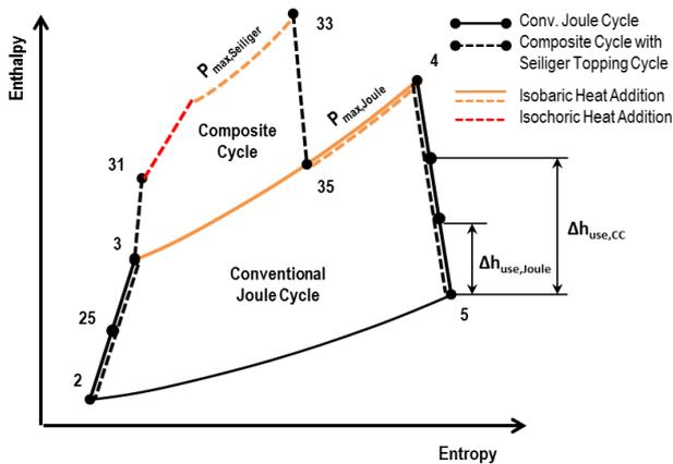
FIG 1. Enthalpy of entropy -diagram of the Composite Cycle and conventional Joule-Brayton Cycle
