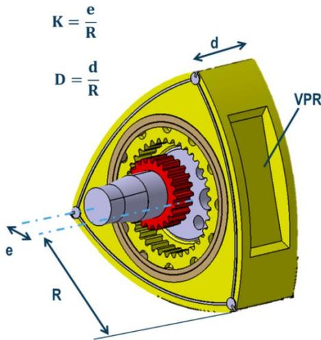
FIG 3. Basic sketch of a rotary engine rotor (yellow) with power shaft (grey) and key geometry parameter (based on [11])
