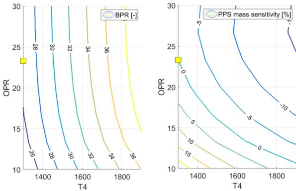
FIG 8. Bypass Ratio (left) and Power Plant System mass sensitivity (right) for  $T_4$ -OPR study
