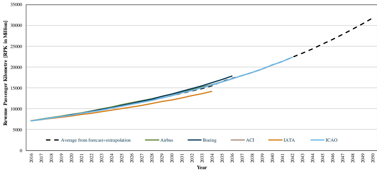
Figure 1: Summary of five different aviation forecast up to the year 2040, average growth function as well as extrapolation up to the year 2050.
