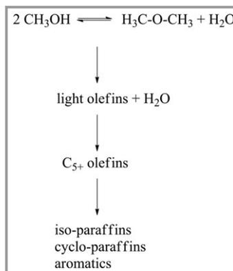
**Figure 5.** Basic process scheme of Mobil’s distillate fuels production from methanol: Light olefins form in a mixture of methanol and dimethylether (DME), further growing to higher olefins, followed by oligomerization to higher branched or cyclic species and mild hydrotreatment, yielding branched (iso) and cyclic paraffins as well as aromatic compounds [50].
