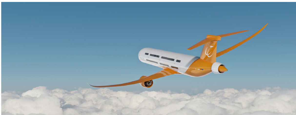
Aircraft concept with boundary layer ingesting propulsor at the aft-fuselage
