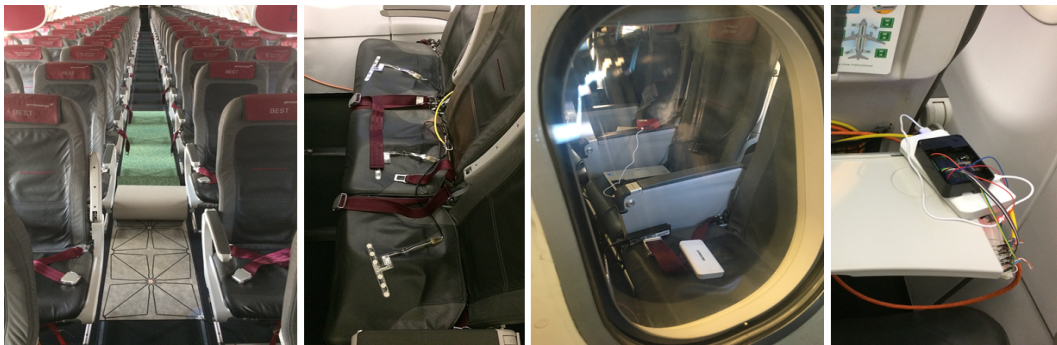
Fig. 9 Sensor environment in a field trial: sensor floor, seat sensors, central processing unit, seat processing unit (from left to right)
