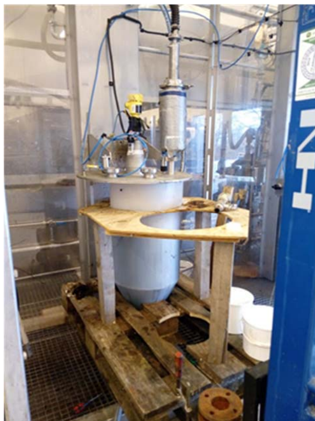
Figure 3: Product collection in the AU HTL pilot plant with hydro-cyclone and separation funnel.
