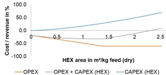
**Figure 6:** Cost optimization for processing sewage sludge via HTL related to a feedstock input of 1 kg sewage sludge (dry).
