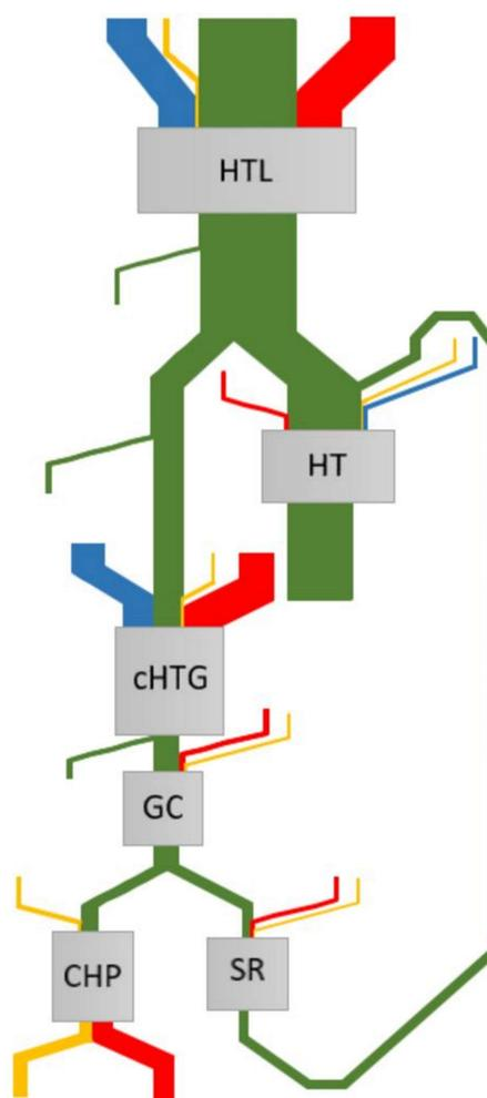
**Figure 5:** Energy balance for an HTL process chain using sewage sludge as HTL feed. Green: Energy in streams, blue: cooling demand, red: heating demand, yellow: electrical power (HTL: hydrothermal liquefaction; HT: hydrotreating; cHTG: catalytic hydrothermal liquefaction; GC: gas cleaning; CHP: combined power and heat plant; SR: steam reforming).
