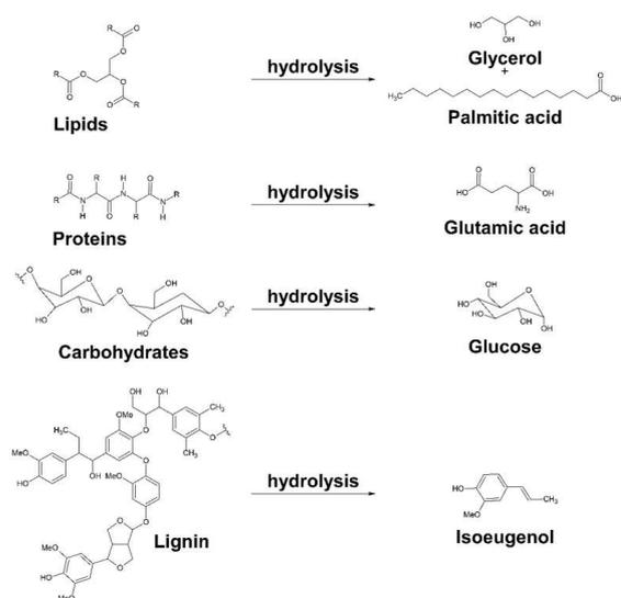
**Figure 2:** Hydrolysis of four biochemical groups for the modelling of the HTL of sewage sludge in Aspen Plus.
