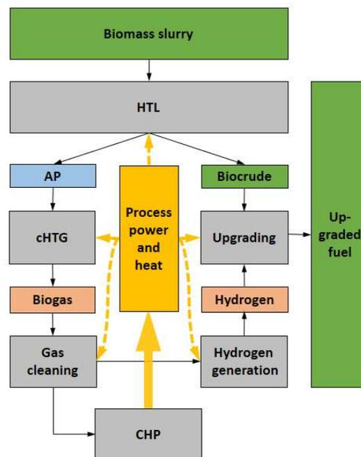
**Figure 1:** Process overview of the modelled and optimized HTL production chain (AP: aqueous phase; cHTG: catalytic hydrothermal liquefaction; CHP: combined power and heat plant).
