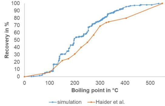
**Figure 4:** Comparison of simulated distillation curves from upgraded biocrude of sewage sludge (blue: model, orange: simulated distillation of upgraded biocrude experimentally produced from sewage sludge) [4].
