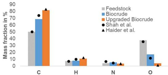
**Figure 3:** Composition of feedstock (grey), biocrude (blue) and upgraded biocrude (orange) using sewage sludge HTL as feedstock [4,12].
