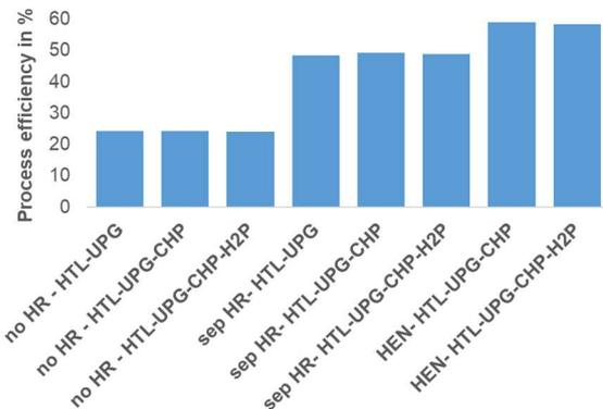
**Figure 7:** Achievable process efficiencies for the configurations considered: no heat recovery (no HR), individual heat recovery in each process step (sep HR), heat exchanger network (HEN).
